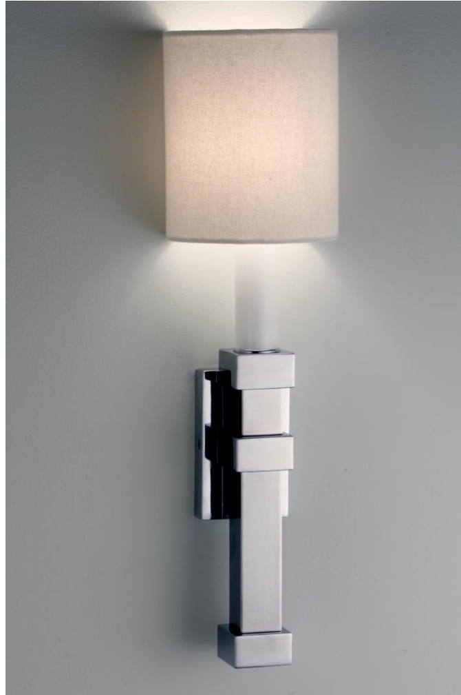
SQUARE COLUMN SCONCE #261EK in Polished Nickel finish (other finishes are available) 17.5" tall x 5" wide 4x " extension 40w. medium base socket off-white linen shade
