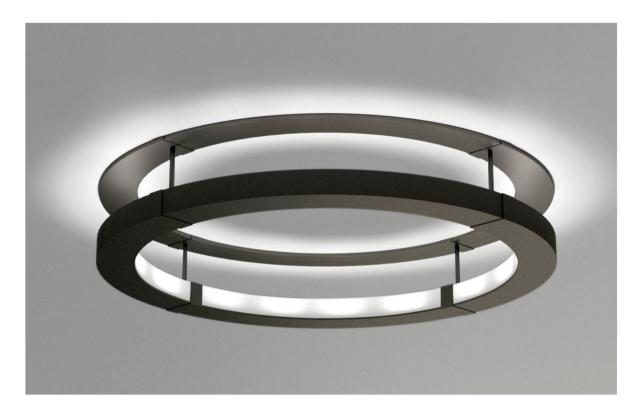
DROP-RING FIXTURE C-815.03 Shown in Dark Oxide painted finish, with opal acrylic diffuser at inner ring. Sixteen medium base sockets for LED bulbs. Mounts to 2" x 3" junction box at perimeter.
