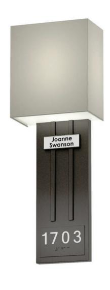
KINGSTON NUMBER SCONCE C-943 20" tall x 7" wide x 4" extension. GU24 socket, UL for 18w CFL or LED bulb. Dark Bronze painted finish, linen shade with opal acrylic diffuser, perforated aluminum screen at top.
