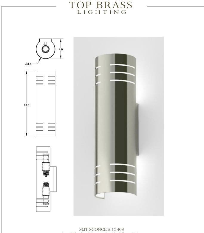
SLIT SCONCE # C1408 in polished stainless steel with diffuser lining, 13" tall x 3.8" wide x 4" extension, 2 x medium base sockets, UL for 10w tubular LED bulbs, Mounts to 2" x 3" rectangle box.
