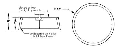
BRAVERN CEILING FIXTURE C1458 18w dedicated LED fixture, 120/277v, 3000K, non-dimming. Dark Oxide finish (ORB39) with champagne finish inside the shade.
