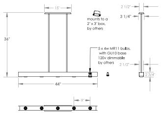
44" wide x 36" overall drop metal with Dark Oxide finish (black) and Polished Chrome around the bulbs 5 x GU10 sockets for MR11 LED bulbs (by others)
