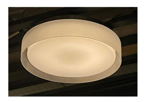
16" diameter x 3.9" drop 24w. LED, 3000K, 2560L delivered 120/277v. driver, triac dimmable steel ceiling pan with matte white paint, frosted outer acrylic and translucent inner diffuser
