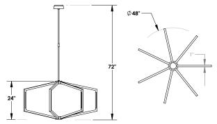
7-Arm LED Chandelier # C2156 48" diameter x 24" tall (main body), 120-277v non-dimming 35w driver, 3000K, 4500L at source Dark Oxide (black) painted finish, silicone diffusers UL/ETL certification
