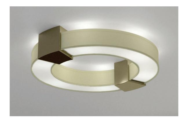
WEDGES CEILING FIXTURE C-827 Shown in Medium Antique Brass finish, with cream linen shade and opal acrylic diffuser. Six medium base sockets for LED or CFL bulbs. Mounts to 4" junction box at perimeter.
